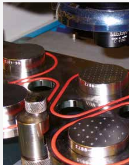
Stage Mensuration of NGI Nozzles using the Mitutoyo QV404 Vision Inspection System
