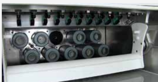
↑ Waste shot collector array
