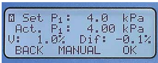
↑ TPK 2100 Display showing Automatic Setting of P1
