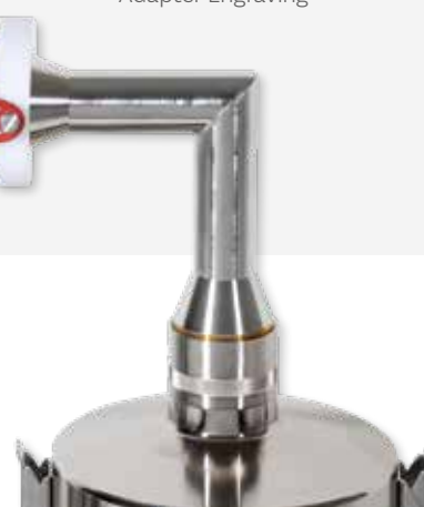
↑ Induction Port with Diskus® Mouthpiece Adapter and Inhaler Support Accessory
