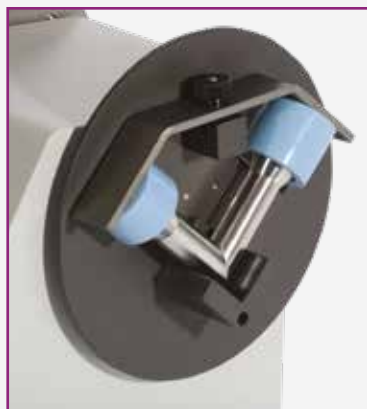
↑ Fixture with NGI Induction Port
