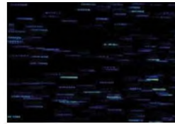
Fringes generated from the droplets in GSV of the droplet size measurements
