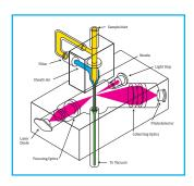
light relative to the amount of aerosol in the air stream. The scattered light is collected by two aspheric lenses and is focused onto a photodiode detector, allowing the user to obtain the relative concentration measurement.
