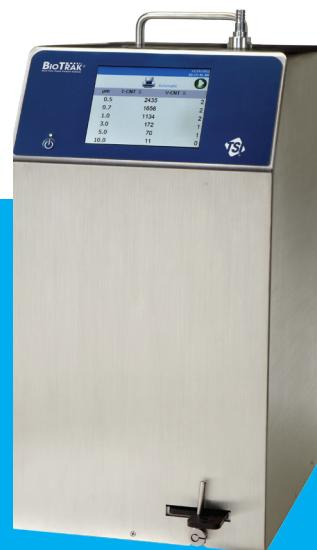
BioTrak® Real-Time Viable Particle Counter offers best-in-class features and versatility in the exciting new field of real-time airborne viable particle detection. The BioTrak particle counter detects total and viable particle counts in real time and incorporates TSI field-proven, patented Laser Induced Fluorescence (LIF) technology to determine particle viability.
