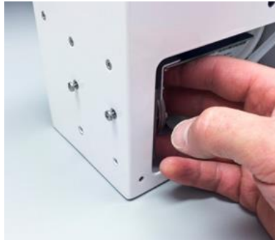
Figure 31: Secure new pump
