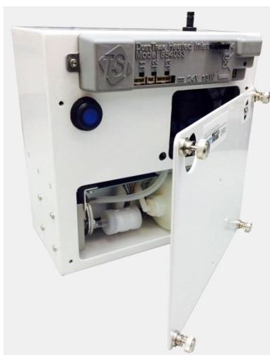
Figure 26: Open instrument service panel
