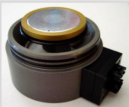
Figure 2. Typical stage with uniform deposit
