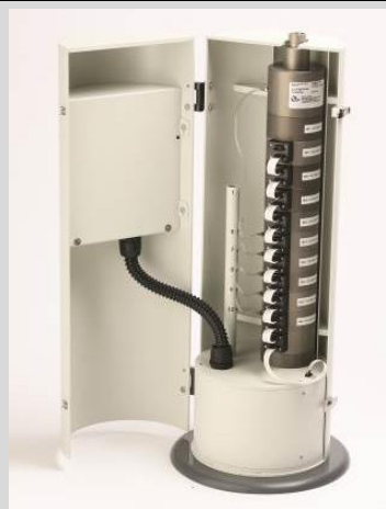
Model 120R 30 L/min 10 Stage MOUDI II impactor
