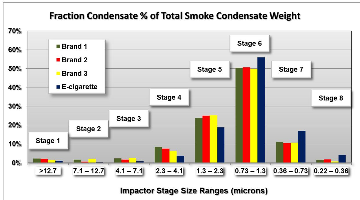
These results show how the Mini-MOUDI impactor enables determination of the aerosol mass contained in various particle size ranges. Further analysis of the samples collected on various Mini-MOUDI stages will reveal the distribution of chemicals, e.g., nicotine and tobacco-specific nitrosamines, in various size bins, providing valuable data concerning the access of the cigarette smoke contents to various regions of the smokers' lungs.
