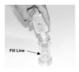
4. Squeeze alcohol into the Alcohol Fill Capsule until it is even with or slightly above the scribed fill-line near the base. RECAP THE ALCOHOL BOTTLE IMMEDIATELY.
