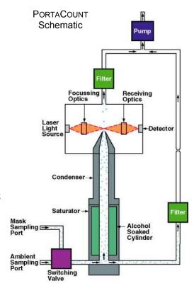
The PORTACOUNT Plus grows submicron particles to supermicron alcohol droplets and then measures the concentration of the alcohol droplets. This makes the PORTACOUNT Plus sensitive to particles having diameters as small as 0.02 microns, but insensitive to variations in particle size, shape, composition, and refractive index. Thus, quantitative fit testing can be performed with virtually any aerosol, including ambient air.
