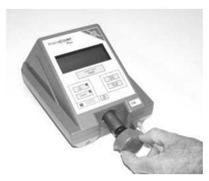
ALWAYS RECAP ALCOHOL FILL CAPSULE AND OTHER CONTAINERS IMMEDIATELY TO PREVENT ABSORPTION OF MOISTURE AND THE ESCAPE OF ALCOHOL VAPORS.
