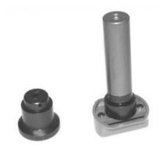
3. Open a bottle of alcohol. Invert the bottle and insert the nozzle end into the Alcohol Fill Capsule as far as possible to make certain that you cannot inadvertently spray alcohol anywhere except down into the Capsule.
