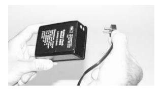
Plug the battery charger into an AC outlet. Be certain that the outlet is the proper voltage for the charger (115 VAC or 220 VAC). Allow the battery to charge for at least 6 hours.
