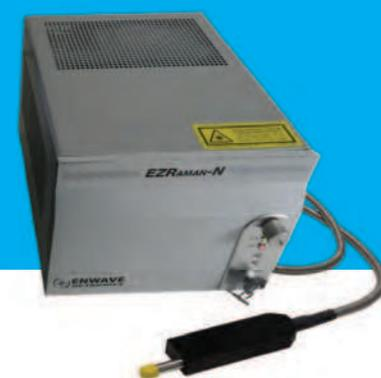
The EZRaman-N system features a narrow linewidth frequency stabilized laser, high throughput fiber optics probe, and an optically fast (f/1.6) spectrograph with TE cooled CCD detector. This system is easy to use with powerful and user-friendly RamanReader software, while providing excellent long term reliability with minimal maintenance.
